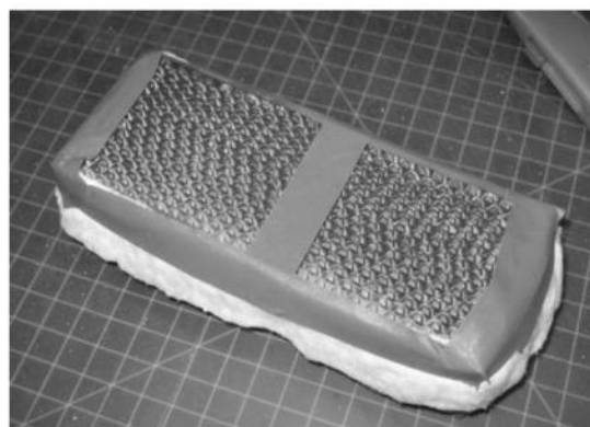
Figure 20 - Installing Gasket on Catalyst
