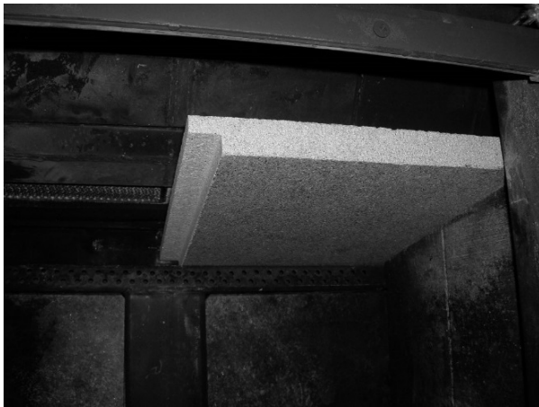
Figure 18 (cont.) - Removing/Replacing the Baffle for Inspection
