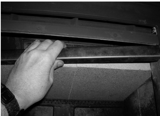
Figure 16 - Removing/Replacing the Baffle for Inspection
